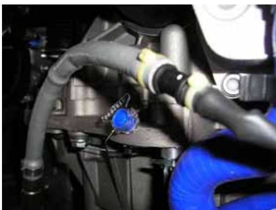
Top transmission seal.
