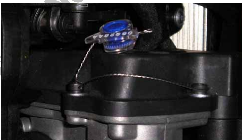
(x) Throttle body seal.
