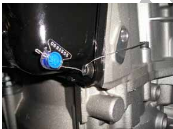
Bottom transmission seal.
