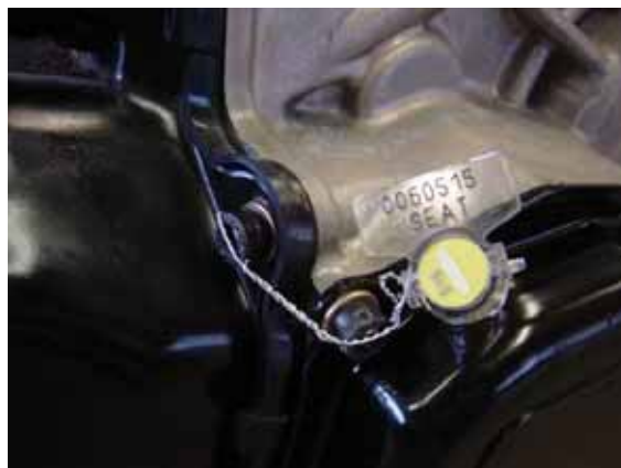
Transmission SEAT Spain seal.
